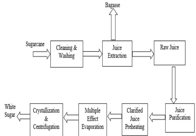
Figure 2: A simplified process diagram for the generation of sugarcane bagasse [17].
